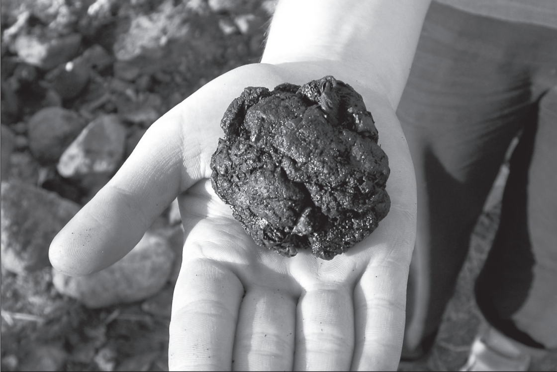
Photo 6 The wood tar made during the course of this experiment was strongly contaminated with charcoal and the remnants of untransformed birch bark. ■
