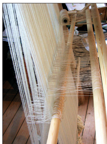
■ Fig. 13 Knitting the heddles. Here, we also see the three shed sticks. The fourth shed is the natural shed.
