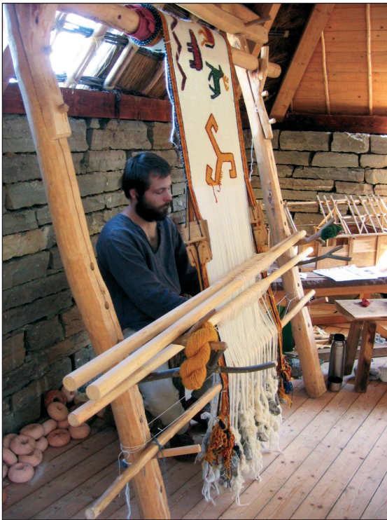
■ Fig. 16 All four sheds of the loom can be seen here.
