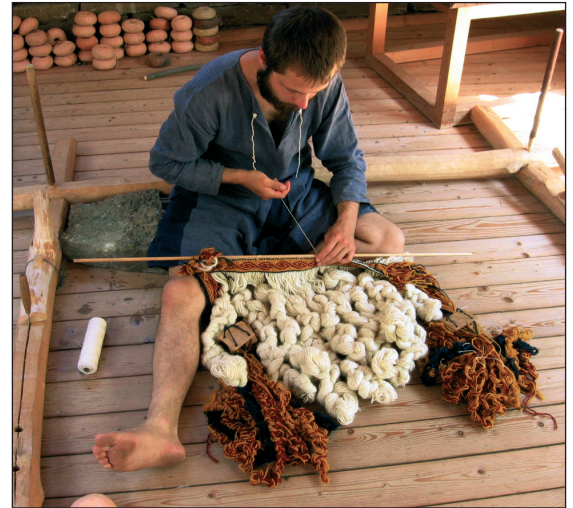
■ Fig. 3 Jan Rodina is sewing the warp to the beam.
