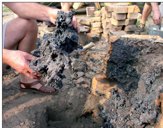
■ Fig. 5 View of achieved slag block in II test
