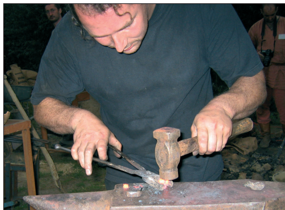
■ Fig. 6 View of the small pieces of iron forging process
