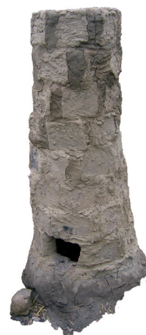
■ Fig. 2 View of the second bloomery furnace
