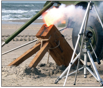
■ Fig. 3 The Loshult gun is fired with a lead ball and 20 grams of gunpowder. The ball reaches 1050 meters. Everything is documented by Military radar
