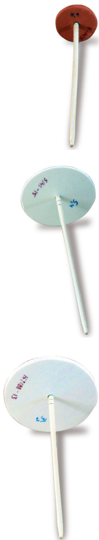
■ Fig. 5 Spindles with clay and plywood whorls used in the experiment. Top reference spindle, whorl 15 g and MI 41, middle whorl 5 g and MI 41, bottom whorl 15 g and MI 188
