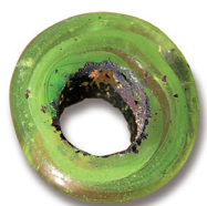
■ Fig. 23 Salt from a saltstone worked very well as a separator. The salt reacted with the iron of the mandrel and left black metallic-like rests in the beadhole
