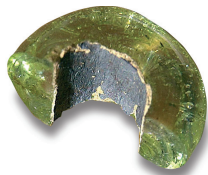
■ Fig. 21 Local clay from the surroundings of Eketorp, Öland did not work well as a separator. The clay stuck to the mandrel and thus made it impossible for me to get the bead off
