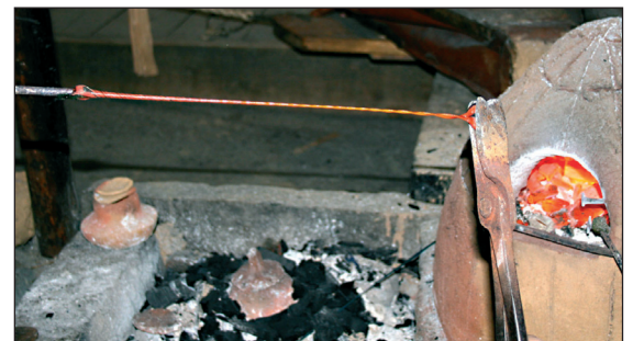
■ Fig. 13 The glass lump with the four monochrome rods is pulled out and twisted until a long “peppermint stick like” rod is created.
