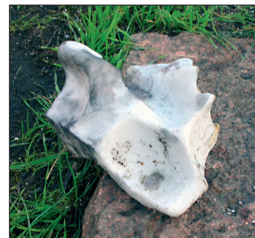
■ Fig. 20 The mandrels were provided with salt from a saltstone. The salt reacted with the iron and worked excellent as a separator
