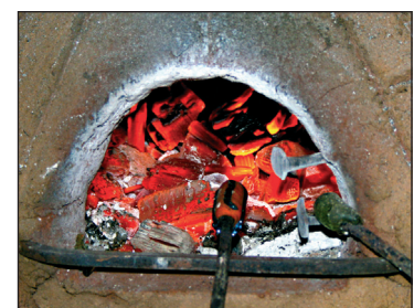
■ Fig. 12 The glass lump with four monochrome glass rods is heated up in the oven
